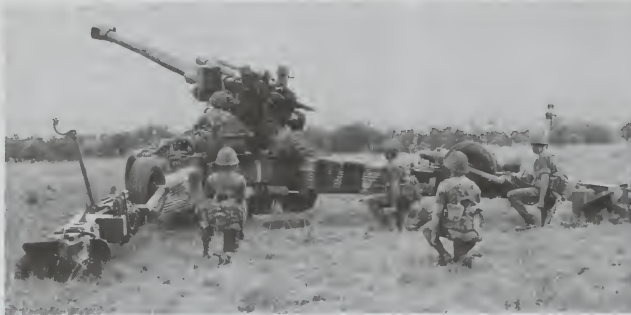
Figure 16: The 155-millimetre South African G5 of 1983. With a computer terminal for displaying gun-laying data and a diesel-fueled auxiliary power unit for opening the trail legs and raising the firing platform, this gun-howitzer epitomized artillery of the late 20th century.
